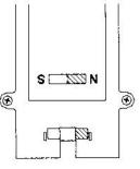
Polarity of the Color Marked Magnet must correspond to the Imprint
